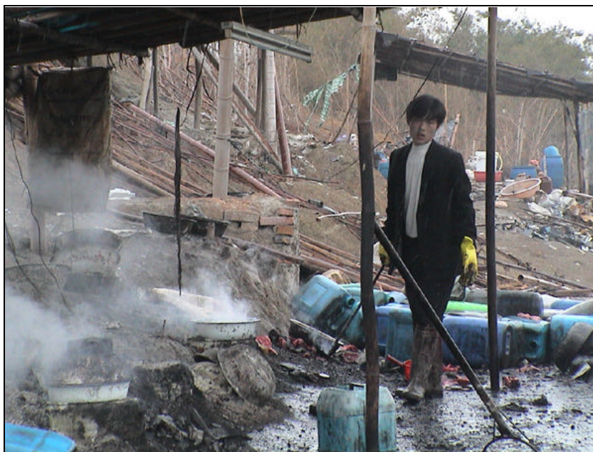
Laborer heating aqua regia – a mixture of 25% pure nitric acid and 75% pure hydrochloric acid – a mixture that will dissolve gold. Without any respiratory protection workers inhale acid fumes, chlorine and sulphur dioxide gas all day as they swirl computer chips removed from circuit boards in acid to collect tiny amounts of gold. The sludges from the process are dumped directly into the river. Guiyu, China. December 2001. © BAN
