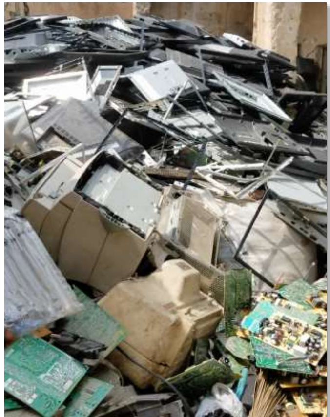
CRT and LCD breakdown site in Peshawar. Contamination by mercury and CRT phosphors, and leaded glass appears as a likely result of this type of operation. Copyright BAN, Shakila Umair, 2018.
