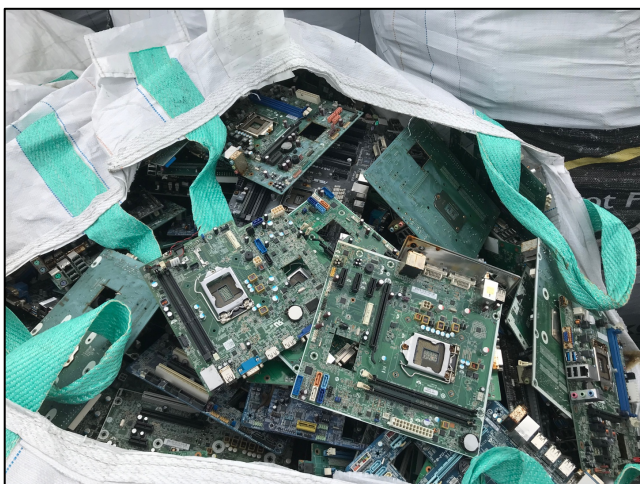
Close-up of circuit boards showing CPUs and gold-bearing chips cut out for aqua-regia processing. These remaining boards will be smelted for copper content. Copyright BAN, July 2018.
