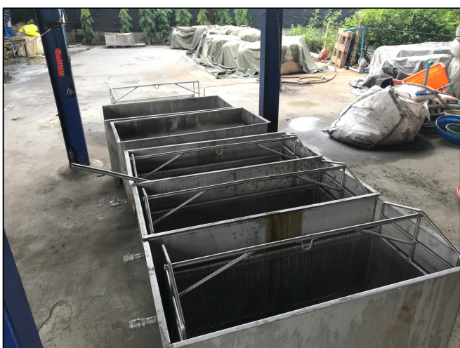
Stainless steel acid tanks and racks for aqua-regia processing of gold-bearing chips. Copyright BAN, July 2018.
