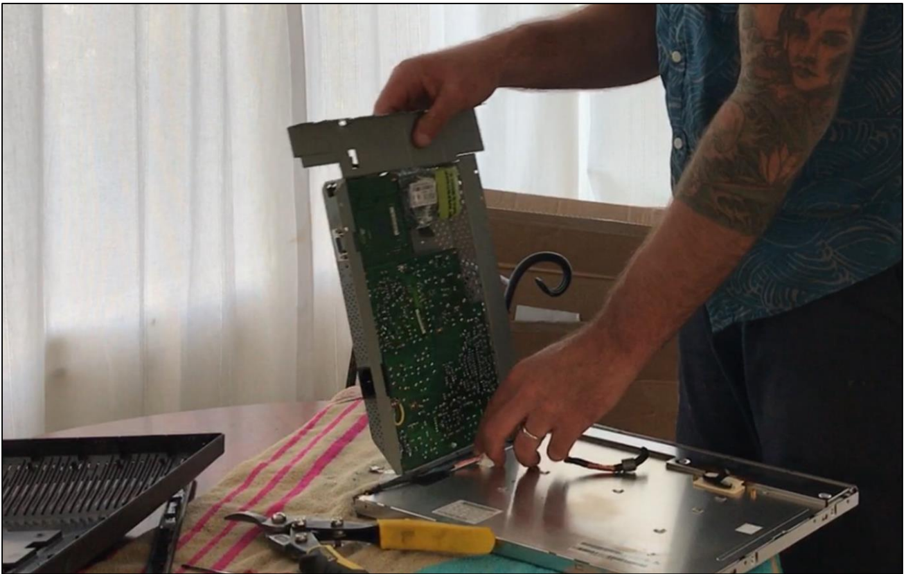
Installation video of tracker in the LCD. See tracker in plastic wrap in upper part of board. Copyright BAN, September 2017.
