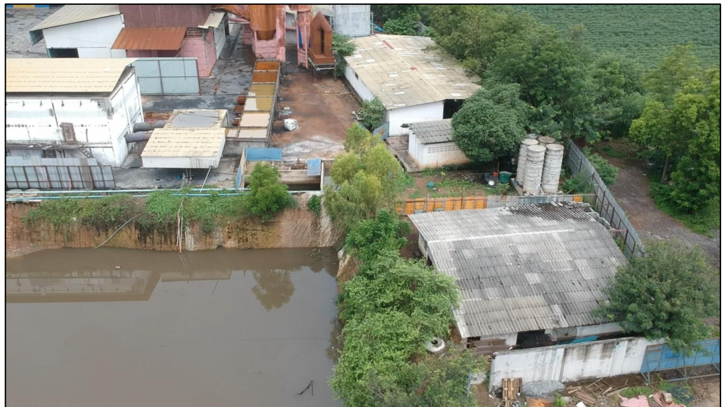
Drone view of aqua regia plant showing stainless steel acid tanks and sludge pond at groundwater level. Copyright BAN, July 2018.
